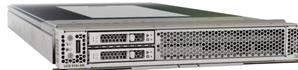
UCS X210c / X215c Compute Node – GPU Up to two on-server GPUs
